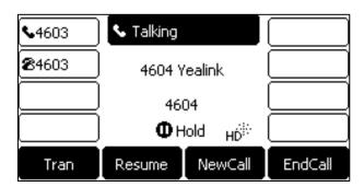
The line key LEDs on phone A slow flash green and phone B slow flash red when the shared line call is placed on hold.
