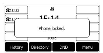
To unlock the phone, you must know the phone unlock PIN. The default phone unlock PIN is "123".
