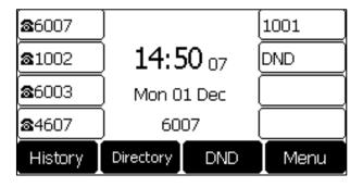
When you assign functionality to line key located in line key 9-21, the label of the line key 8-14 are indicated on the second page, and the labels of the line key 15-21 are indicated on the third page. The line key in the right bottom is used to switch pages. The following figure shows an example:
