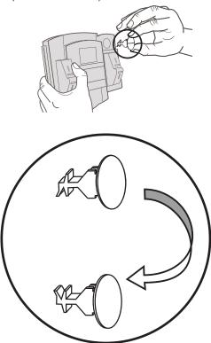
**6.** Re-insert the hookswitch tab, and then push it into a locked position, using your thumb. The hookswitch tab is now in "wallmount" position.
