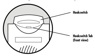
Your SoundPoint IP phone is packaged with the hookswitch tab in "deskmount" position. Before your phone can be mounted to the wall, the hookswitch tab must be set to the "wallmount" position.
