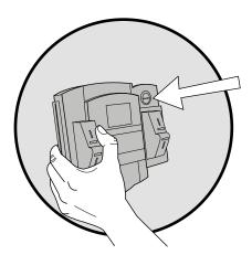
**2.** Using your thumb or forefinger, push the tab downward.
