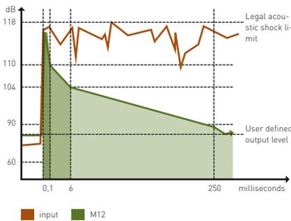
Figures given are with midpoint volume setting 5. All limiting-levels track up and down with the volume setting, so loud noises are clamped at higher sound levels than those described above for higher volume settings, and at lower sound levels for lower volume settings. The volume control has a total adjustment range of 21dB.
