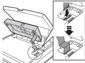
4. Connect the USB cable to the USB port.
