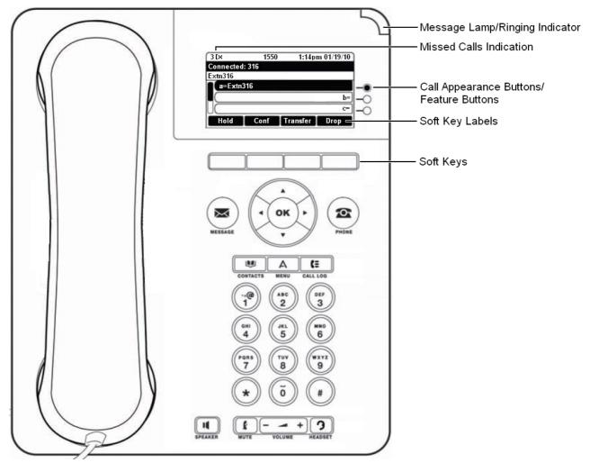
This phone supports 12 programmable call appearance/feature buttons. The labels for 3 of these buttons are visible on the main display and can be controlled by the adjacent buttons to the right. You can use the  $\blacktriangle$  up and down  $\forall$  arrow keys to scroll the display. You can also use the  $\blacktriangleleft$  left and right  $\blacktriangleright$  arrow keys to move through the button features in pages of 3.
